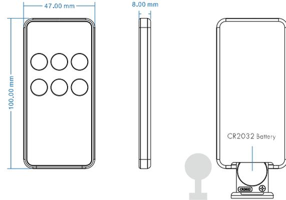
**Note:** Before the first use, please remove the protective film on the battery.
